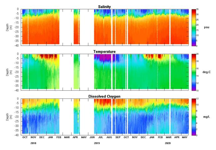
Figure 6 Observations from the CSIRO profile mooring at King River Basin site (Figure 2) showing the temporal change of water column salinity, temperature and dissolved oxygen concentration from October 2018 to May 2020. Profiling operations were suspended (i.e. the gaps in the figure) during very rough weather to avoid entanglement, and on a few occasions to enable platform maintenance.
